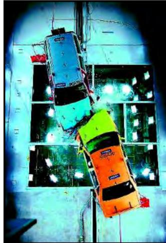
The effect of this crumpling is to increase the time ( $\Delta t$ ) for the car to come to rest when it is involved in a collision. According to Newton's second law,  $F = \Delta(mv)/\Delta t$  and so for a given momentum decrease  $\Delta(mv)$ , an increase in the impact time ( $\Delta t$ ) means a decrease in the impact force ( $F$ ) which acts on the car and passengers.
