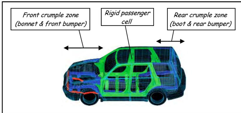
Other parts of the car, such as the **passenger cell**, are designed as a very strong, rigid compartment so as to maximise passenger protection in the event of a collision.
