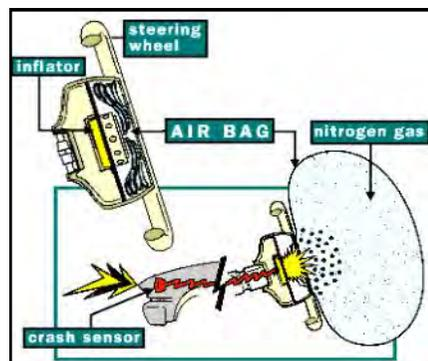
\* The **accelerometer** consists of two rows of interlocking teeth which will move relative to each other when subjected to the large deceleration produced in a collision. This movement generates a voltage which is used to trigger the inflation of the air-bag.
